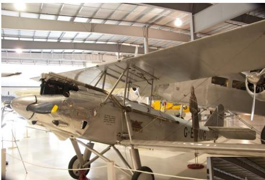
Early airplane designers worked on both monoplane and biplane concepts in development of design based on technology available. Their efforts centered on making wings capable of withstanding the required loads. Considering the technology of the day, the biplane could be made lighter for a given strength requirement, and was the common choice. Most aircraft built between 1914 and 1925 were biplanes using the same box kite design concept as the Wright Flier designs.
