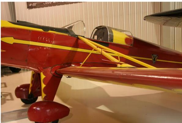
A **low wing** design places the lower surface of the wing level with the bottom of the fuselage. A **mid-wing** places the wing mid-way on the fuselage. A **shoulder wing** is placed above the center on the fuselage. A **high wing** design places the wing with the wings upper surface level or above the fuselage. The **parasol wing** design places the wing above the fuselage and is not connected directly but will have struts and wires for attachment to the fuselage,
